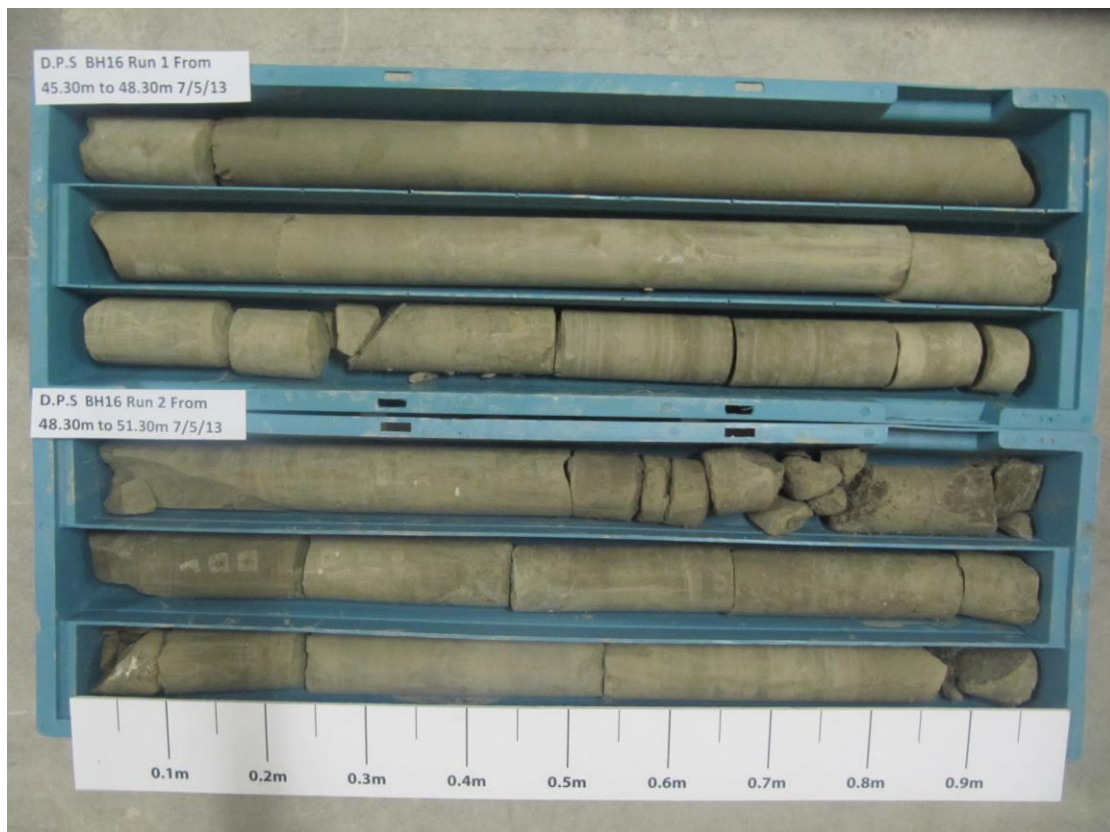
Plate 11: Core samples recovered from BH16 Run 1 and Run 2
