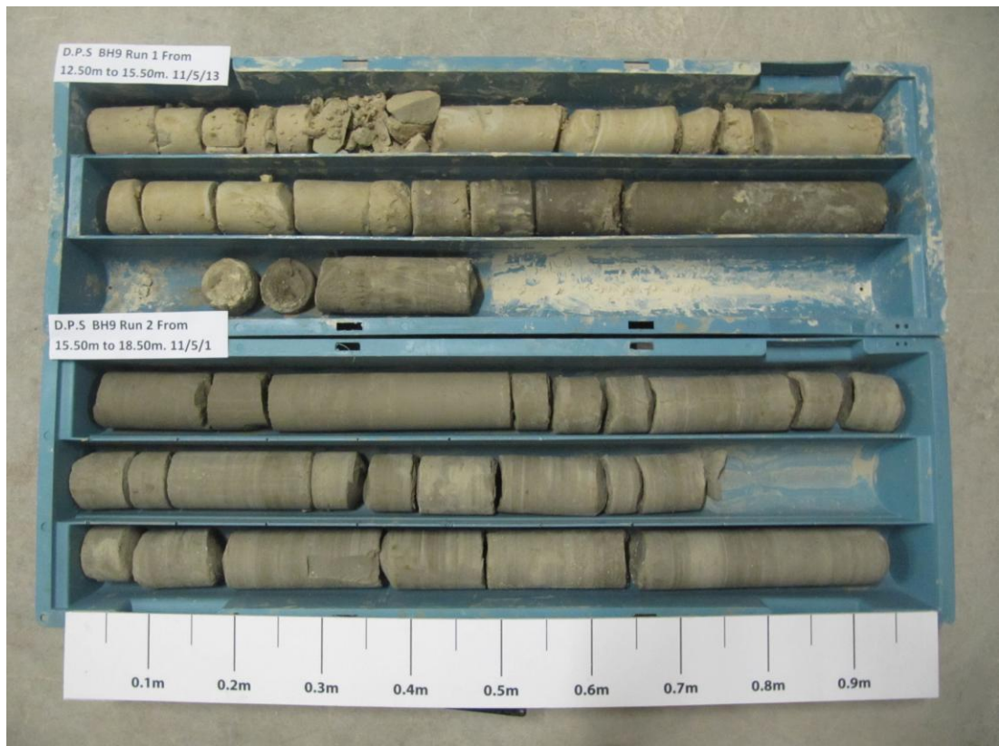
Plate 8: Core samples recovered from BH9 Run 1 and Run 2
