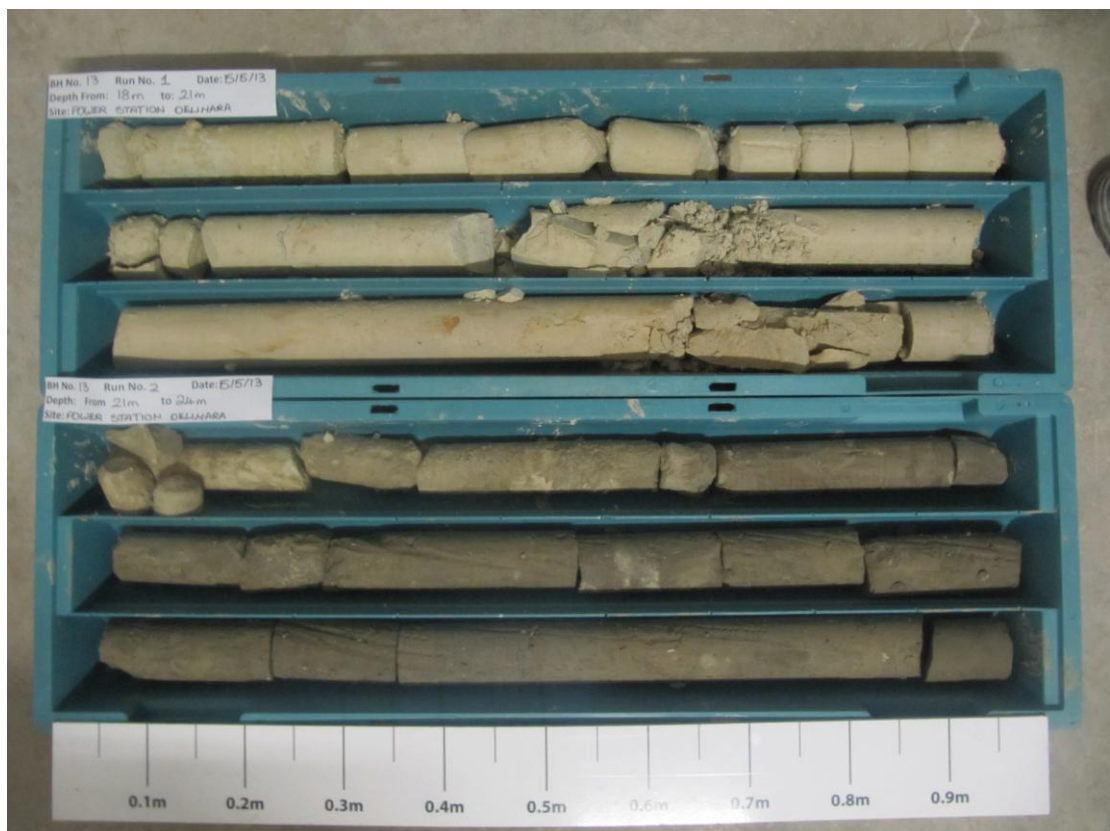
Plate 8: Core samples recovered from BH9 Run 1 and Run 2
