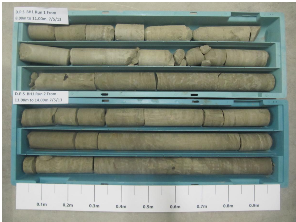
Plate 1: Core sample recovered from BH 1 Run 1 and Run 2
