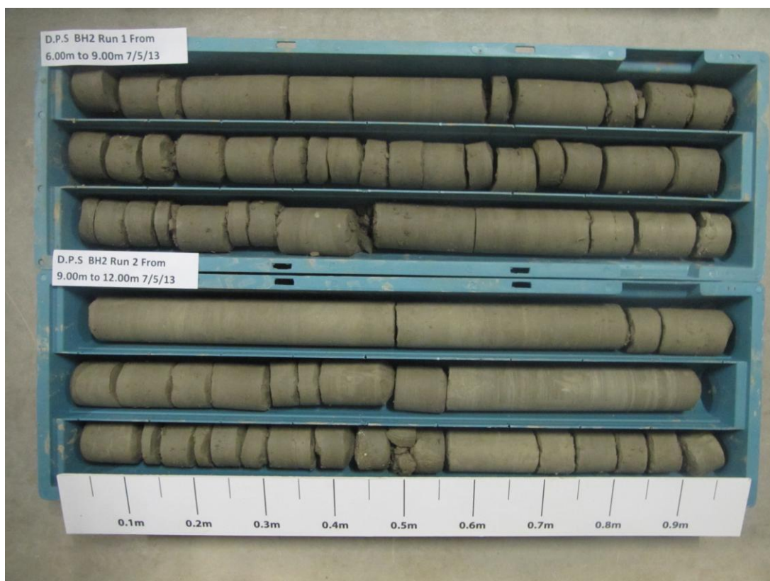
Plate 2: Core samples recovered from BH 2 Run 1 and Run 2
