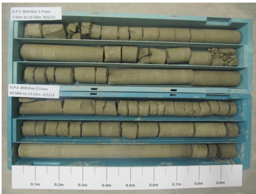
Plate 4: Core sample recovered from BH4 Run 1 and Run 2
